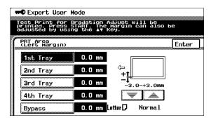
9 Check that the left margin of the test pattern is between 2.5 mm and 3.5 mm. If the left margin is within the specified range, skip to step 14.
